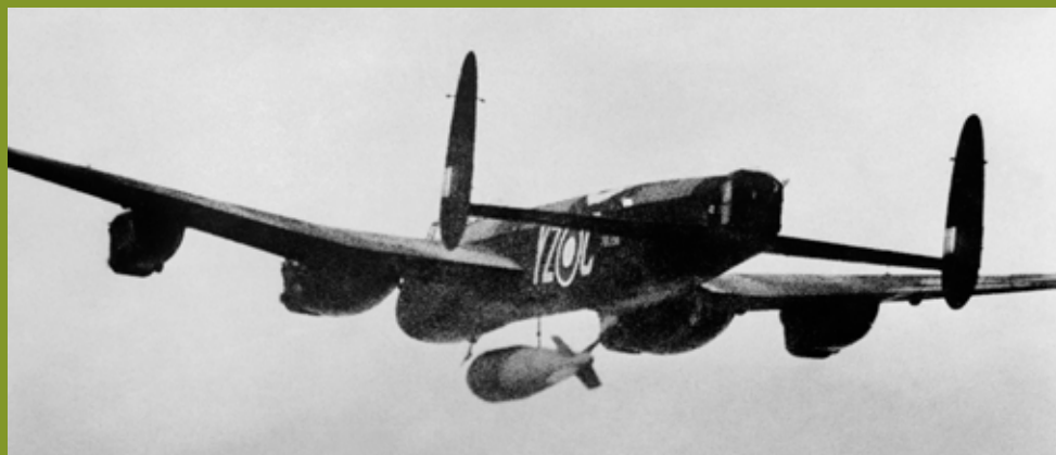
A 12,000 lb Tallboy bomb being dropped by a Lancaster B Mk. I (Special). The bomb was so big only one could be carried. Photo: Crown Copyright (Public Domain).
