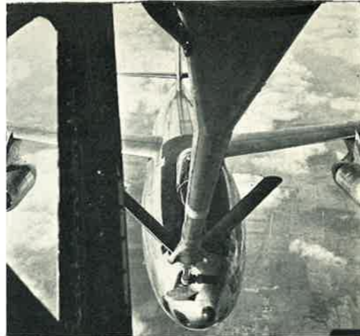
A view from 'Clancy's' position in a U.S.A.F. KC-97 tanker of the refuelling boom lowered and in action. While the U.S.N. and Tactical Air Command have adopted the probe and drogue system, Strategic Air Command has opted for the celebrated Boeing boom.
