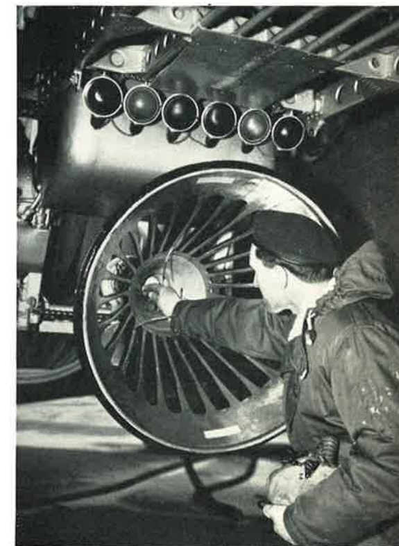
Close-up of the H.D.U. on a Valiant, showing the drogue and six signal lights by which the tanker communicates with the recipient.
