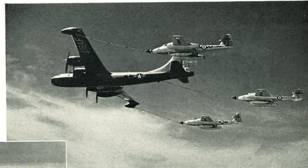
Above: In 1951, 16 Meteor 8s of No. 245 Squadron, Horsham St Faith, were fitted with flight refuelling nose probes for R.A.F. evaluation trials. While they were proceeding, Flight Refuelling Ltd began three-point trials for the U.S.A.F. with a B-29, and the 245 Squadron Meteors co-operated - as is shown in this picture taken over the Norfolk coast near Cromer.
