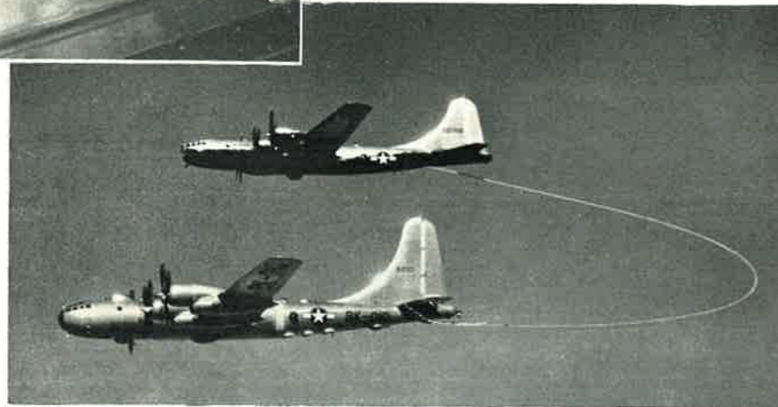
Right: "Lucky Lady II", the U.S.A.F. B-50 which, in 1949, sustained by flight refuelling, made a non-stop round-the-world flight of 94 hours continuous flying. In this picture, taken on a training flight beforehand, "Lucky Lady" is being refuelled over Arizona by a B-29 tanker - again the looped hose method.
