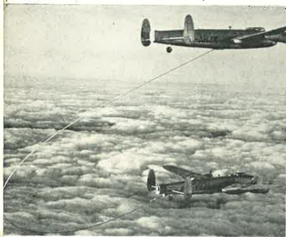
Above: Lancaster-to-Lancaster looped hose trials conducted by Flight Refuelling Ltd in 1946. Because this system called for an operator in the receiver aircraft it could not be used for fighters. The probe and drogue method overcame this limitation and the looped hose technique is no longer used.
