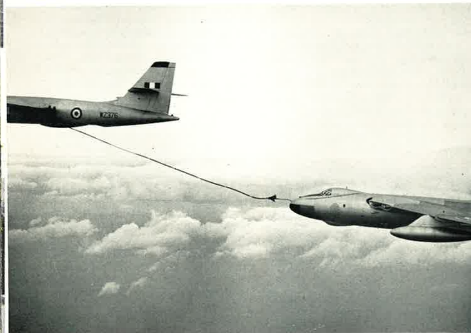
"When a contact has been made... a little power may be applied to move sedately and under perfect control up into the refuelling position."
