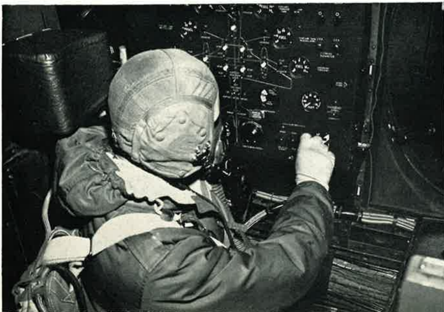
Above: Valiant feeds Valiant. Below: Key man in the Valiant tanker, the panel operator. Lights on the panel give such a full picture of refuelling progress that R/T conversation is normally unnecessary. The operator here is Flight Sergeant K. Symonds.
