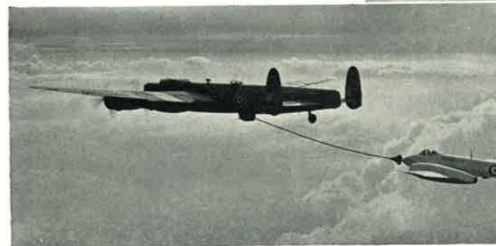
Above: One of the Lincoln tankers used in the 1951 trials with 245 Squadron's Meteors. Right: An eagle's eye view of a United States Navy A.J-1 Savage, a carrier borne tanker, refuelling an F-7U fighter. The U.S.N. has adopted probe and drogue refuelling. So has Tactical Air Command.
